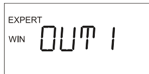
Fig. 63. Output 1 configured as a "WIN" monitor
