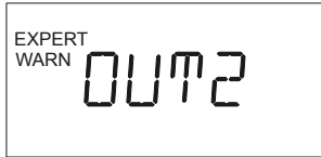
Fig. 64. OUT2 configured as a warning output
