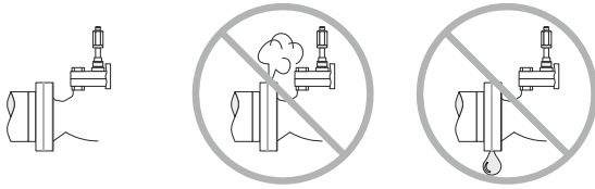
Fig. 2. Piping must prevent leakage
