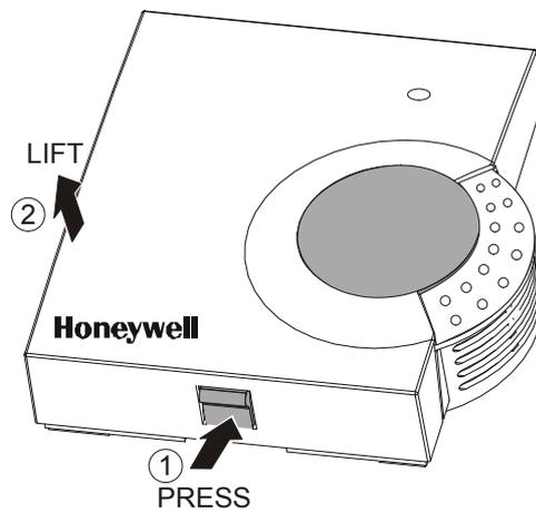
Fig. 2. Cover disassembly
